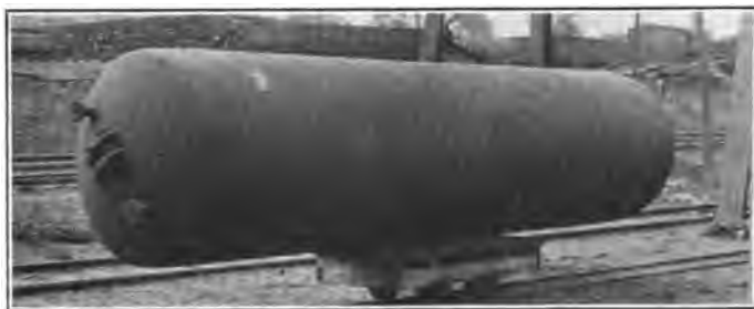
FIG. 144. Pressure tank for storage of hydrogen.
